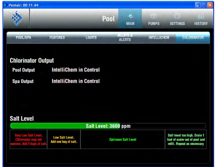
Chlorinator (IntelliChlor) with IntelliChem controller screen
